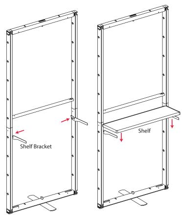
1. Attach two shelf brackets on the inside slots of the frame. Brackets will need to pass through slots in the fabric graphic (not shown above).
