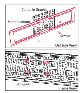
3. Install the fabric graphic with monitor mount cutout aligned over the monitor mount plate. See graphic installation instructions for details.
