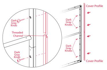
1. To cover the slots at the end of a frame, attach cover profiles with dark gray knobs as seen above. The knobs attach to the cover profile's threaded channel.
