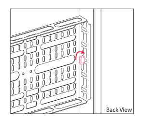
1. Attach the monitor plate to the frame(s) with monitor mount connectors (marked in red). Two plates may be attached on two adjacent frames as seen above. The plate will be flush to the front of the frame(s). Note: Attaching a monitor mount on the front of a room requires different mounting hardware. See the following page for details. 2. Twist the ends of the connectors ninety degrees to lock them in place.
