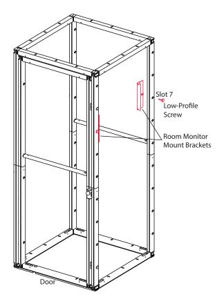
1. Attach two room monitor mount brackets with low-profile screws in slot 7.
