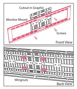
3. Install the fabric graphic with monitor mount cutout aligned over the monitor mount plate. See graphic installation instructions for details.
