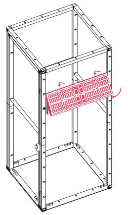
2. Hang the montor bracket plate onto the brackets.
