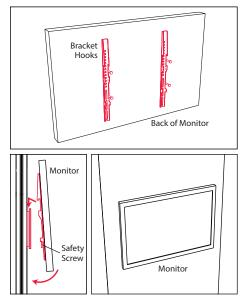
5. Attach the monitor mount hook bars onto the back of the monitor.
