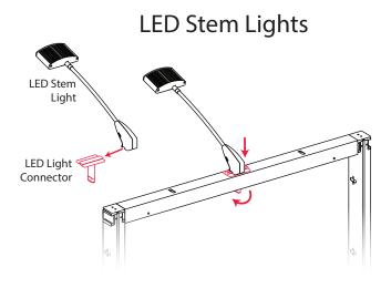
1. Attach the LED Stem Light to the LED Light connector (marked in red).
