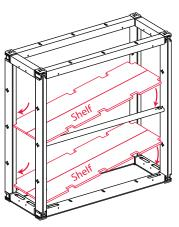
5. Unfold and rest one shelf on the bottom horizontal bars. Unfold and rest the second shelf on the support bars.
