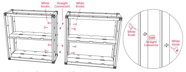
7. Attach the two frames together with four straight connectors. The straight connectors are placed between the frames and are secured with two white knobs each.
