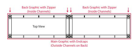
8. Install the fabric graphics. See graphic installation instructions for details. It is most common for the front graphic to start on the back, wrap around the left side, front, right side, and end on the back.
