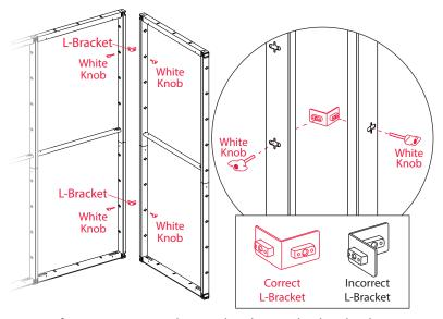
6. To form a corner, attach two L-brackets with white knobs. Note: Constructing a room requires a different L-bracket. See the room assembly instructions for details.
