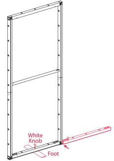
4. Where shown in the kit frame diagram, attach feet to the bottom of the frame with white knobs.
