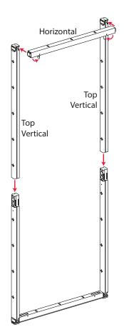
2. Slide the top vertical bars over the bottom vertical bars. Attach the top horizontals and lock their levers.
