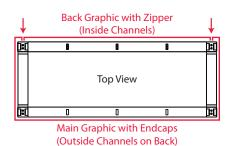
6. Install the fabric graphics. See graphic installation instructions for details. It is most common for the front graphic to start on the back, wrap around the left side, front, right side, and end on the back.
