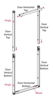
9. Assemble the door perimeter as seen above making sure that the wheel is oriented away from the side with hinges.
