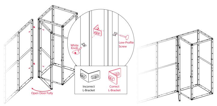
13. To build a wall connected to the room, use two special L-Brackets with opposite connection orientation. Attach each connector to the storage room using a low profile screw and connect to the wall using a white knob as shown to show above.
