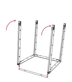
3. Tilt the assembly back and attach the threshold to the bottom of the doorway opening.
