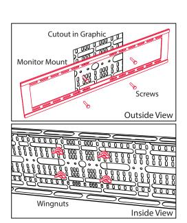
3. Install the fabric graphic with monitor mount cutout aligned over the monitor mount plate. See graphic installation instructions for details.
