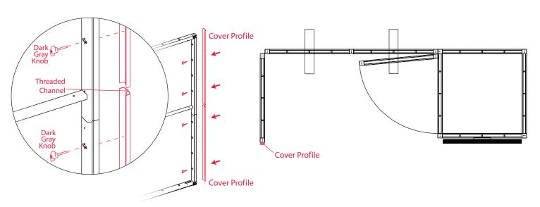
3. To cover the slots at the end the frame, attach cover profiles with dark gray knobs as seen above. The knobs attach to the cover profile's threaded channel.
