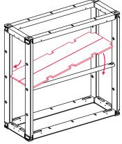
6. Install the fabric graphics. See graphic installation instructions for details. It is most common for the front graphic to start on the back, wrap around the left side, front, right side, and end on the back.
