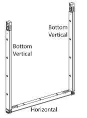
1. Assemble the first frame by connecting one horizontal bar between two bottom verticals, lift the lock levers, slide the parts together, and close the lock levers.
