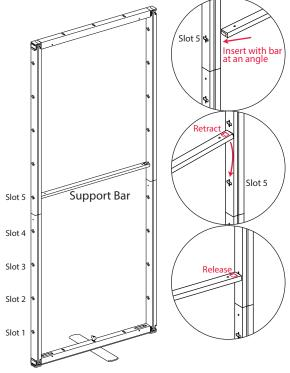
3. Attach the support bar by inserting the non-spring-loaded end into the 5th slot on the left with the other end of the bar lifted. Retract the spring lock and lower the right side until it lines up with the right slot. Release the spring lock.
