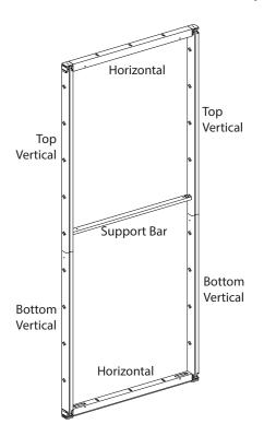
1. Build a frame with two horizontals, two bottom verticals, two top verticals, and a support bar.
