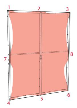
2. Starting in the top/left corner, tuck the graphic. Tuck periodically across the top and then the top/right corner. Repeat for the bottom edge. Tuck the center of the veritical edges.
