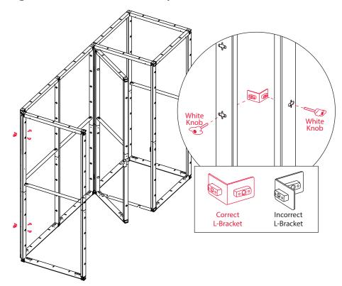
2. Attach the frame to the backwall with two standard L-Brackets and four white knobs as shown above.
