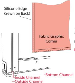
1. To install fabric grahics, turn the edge and tuck the silicone strip into the channel in the frame. The stiched edge goes in first.
