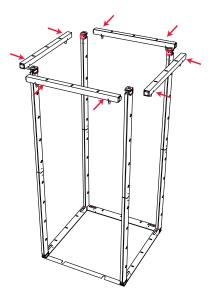
5. Complete the upper half of the storage room by attaching 4 horizontal bars. The levers should be on the bottom of the horizontal bars.
