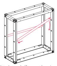
4. Attach two shelf support bars. Insert the non-spring-loaded end into the slot on the left with the other end of the bar lifted. Retract the spring lock and lower the right side until it lines up with the right slot. Release the spring lock.
