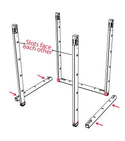
1. Locate two bottom vertical bars with 3-way corners. Attach a horizontal to the bottom between. the verticals Note the direction of the 3-way connectors noted above.
