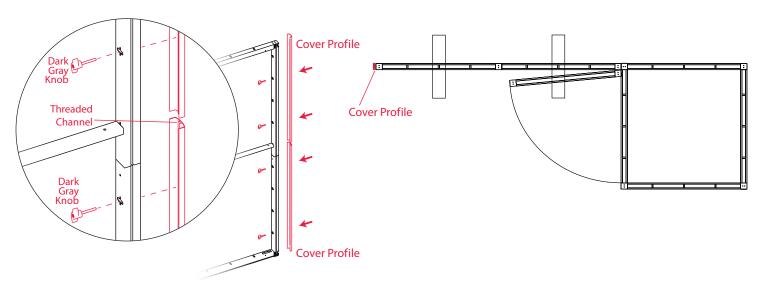
6. To cover the slots at the end the frame, attach cover profiles with dark gray knobs as seen above. The knobs attach to the cover profile's threaded channel.
