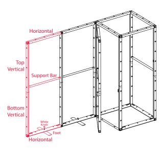
5. Extend the backwall by adding two more horizontals, foot with white knob, bottom vertical, top vertical, and support bar as seen above.
