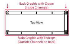
6. Install the fabric graphics. See graphic installation instructions for details. It is most common for the front graphic to start on the back, wrap around the left side, front, right side, and end on the back.
