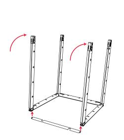
3. Tilt the assembly back and attach the threshold to the bottom of the doorway opening.
