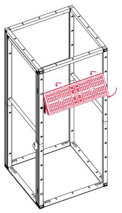
2. Hang the montor bracket plate onto the brackets.
