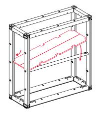
5. Unfold and rest the shelf on the support bars.
