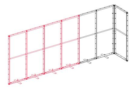
7. Extend the backwall by adding two more horizontals, foot with white knob, bottom vertical, top vertical, and support bar as seen above.
