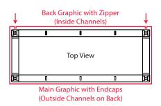
6. Install the fabric graphics. See graphic installation instructions for details. It is most common for the front graphic to start on the back, wrap around the left side, front, right side, and end on the back. 7. Unfold and rest the countertop on top.
