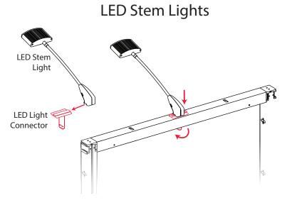
Attach the LED Stem Light to the LED Light connector (marked in red).
