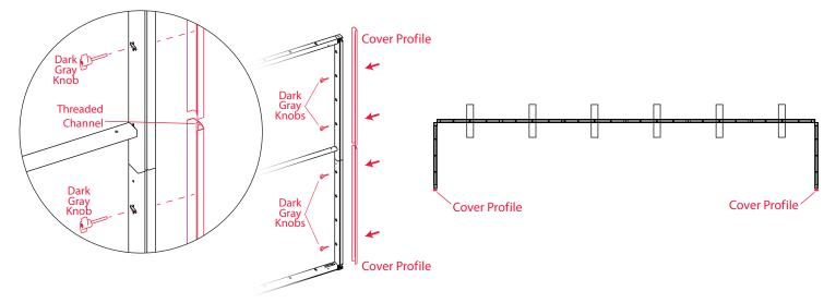
11. To cover the slots at the end of the frames, attach cover profiles with dark gray knobs as seen above. The knobs attach to the cover profile's threaded channel.
