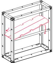
5. Unfold and rest the shelf on the support bars.
