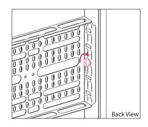
1. Attach the monitor plate to the frame(s) with monitor mount connectors (marked in red). Two plates may be attached on two adjacent frames as seen above. The plate will be flush to the front of the frame(s). Note: Attaching a monitor mount on the front of a room requires different mounting hardware. See the room instructions for details. 2. Twist the ends of the connectors ninety degrees to lock them in place.
