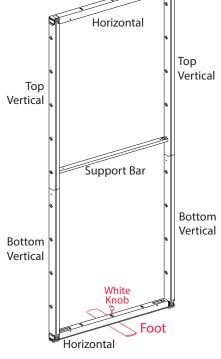
4. Repeat steps 1-3 to build a second frame. 5. Attach a foot to the frame and secure with a white knob.
