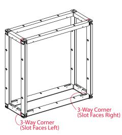
3. Add two more vertical bars, making sure that the short horizontal bars attach to their 3-way corners. Add the remaining horizontal bars to complete the frame. Lock all levers.
