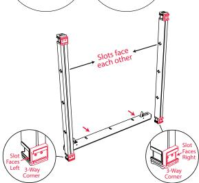
1. Locate two short vertical bars with 3-way corners on both ends. Attach the two together with a horizontal bar by lifting the lock levers and sliding the parts together.
