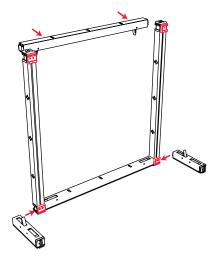
2. Attach two short horizontals to the bottom 3-way corners. Attach a long horizontal to the top of the verticals. Do not lock levers on the small horizontals until step 3.
