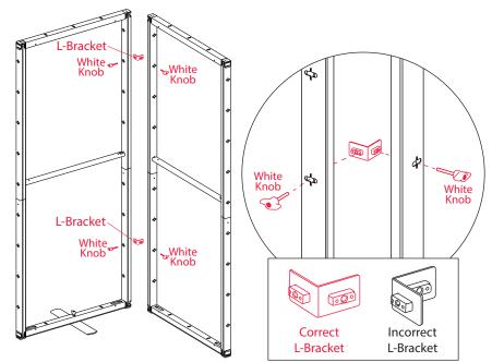
6. Connect the two frames together witht two standard L-brackets and four white knobs. This forms the back/right corner of the display.
