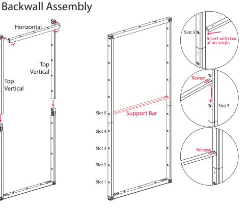
1. Assemble the first frame by connecting one horizontal bar between two bottom verticals, lift the lock levers, slide the parts together, and close the lock levers.
