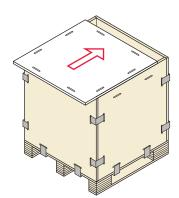
7. Fit top between the 2 sides and slide into place.
