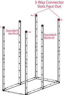
4. Add four upper 3-way verticals as seen above noting the 3-way slot directions. Add standard upper verticals to the two center columns.
