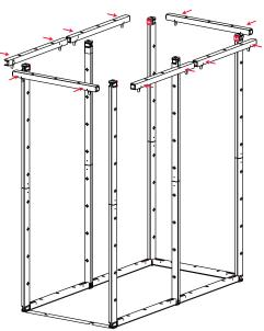
5. Complete the upper half of the storage room by attaching 6 horizontal bars. The levers should be on the bottom of the horizontal bars.
