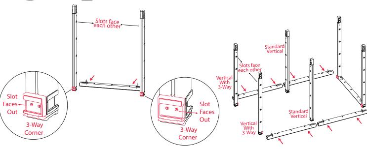
1. Locate two bottom vertical bars with 3-way corners. Attach a horizontal to the bottom between. the verticals Note the direction of the 3-way connectors noted above.
