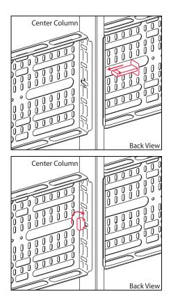
3. Insert a straight connector through the two monitor brackets and the column between. Twist the ends of the connector ninety degrees to secure.
