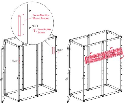
1. On the outer two columns, attach two room monitor mount brackets with low-profile screws in slot 7.
