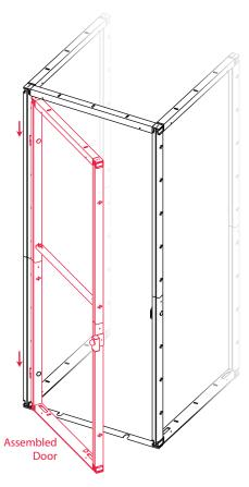
12. Hang the door on the hinges. It is easiest to slide door on hinges when you position door vertical parallel to the storage vertical.
