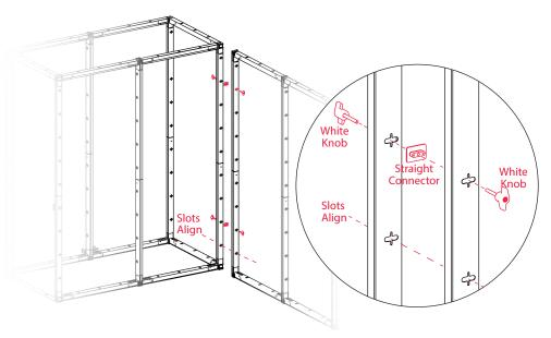
To build a wall connected to the room when the slots align, use two straight connectors. The straight connectors are placed between the frames and are secured with two white knobs each.
