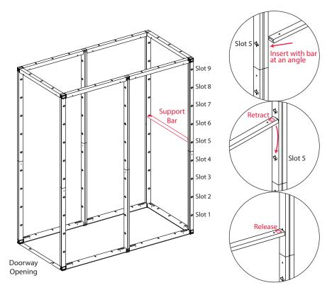
6. Attach a spring-loaded support bar to the wall opposite the doorway in slot 5.
