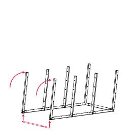
3. Tilt the assembly back and attach the threshold to the bottom of the doorway opening.
