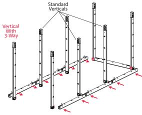
1. Locate two bottom vertical bars with 3-way corners. Attach a horizontal to the bottom between. the verticals Note the direction of the 3-way connectors noted above.
