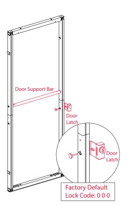
10. Attach the door support bar in the slot above the seam in the vertical bars.
