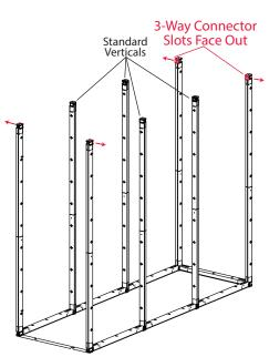
4. Add four upper 3-way verticals as seen above noting the 3-way slot directions. Add standard upper verticals to the four center columns.
