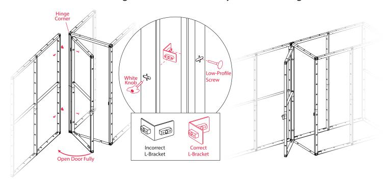
To build a wall connected to the room on the door hinge corner, use two special L-Brackets with opposite connection orientation. Attach each connector to the storage room using a low profile screw and connect to the wall using a white knob as shown to show above.
