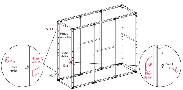
7. Attach the hinges with pins facing upwards on the left side of the doorway in lots 1 and 8 using low-profile screws.
