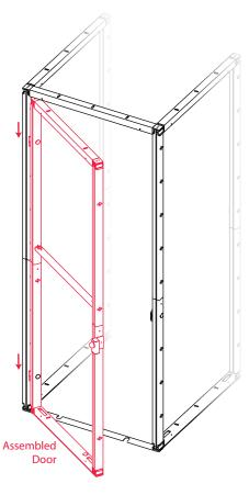
12. Hang the door on the hinges. It is easiest to slide door on hinges when you position door vertical parallel to the storage vertical.
