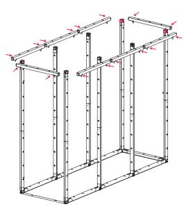
5. Complete the upper half of the storage room by attaching 8 horizontal bars.
