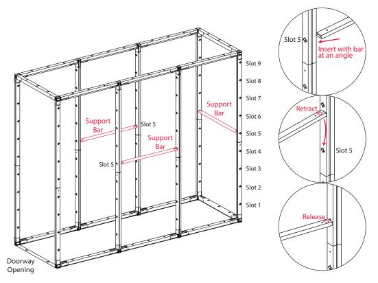
6. Attach spring-loaded support bars in the locations seen above.
